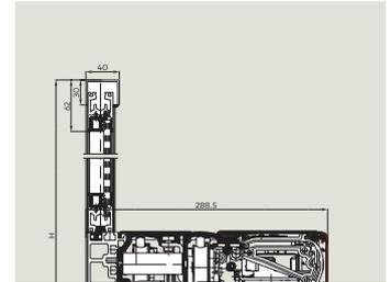
Corridor mounting with side screens, operator 100 mm
