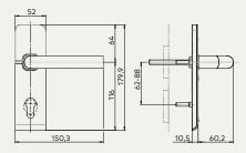
c-lever air, standard version, type 2944 (wide) and 2924 (narrow) Display of EU cylinder profiles (continuous line) and Swiss round profile (dashed line)
